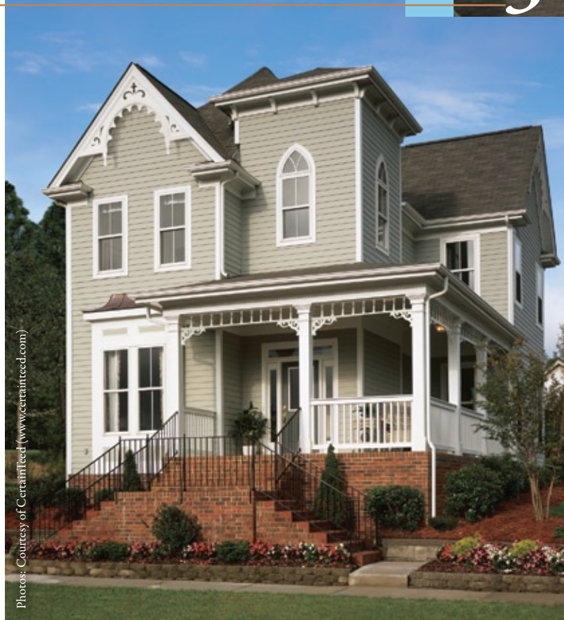
CertainTeed's Restoration Millwork Exterior Trim is made from easy-care PVC, but looks and feels like lumber.
